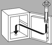
GB The safe must be anchored when in use.
