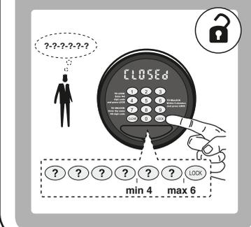
GB To check that your PIN code has been accepted operate the lock three times without closing the door. If unsure repeat the steps above.
